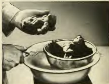
4. Soften clay so it will be easy to "work" by keeping it in hot water in a double boiler—or sieve and warming pan, as shown.
